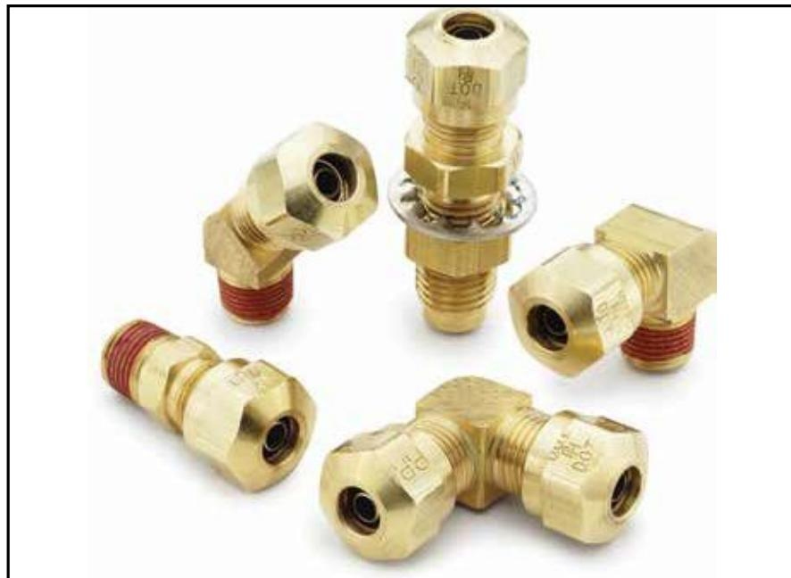
Fittings meet D.O.T. FMVSS 571.106 air brake specifications. Fittings utilize a ribbed sleeve for compression and positive grip. Fittings are pre-applied with thread sealant. Meets functional requirements of the SAE automotive tube fitting standards: SAE J246 and SAE J1131. Electroless nickel plated bodies can be used with bio-diesel.
